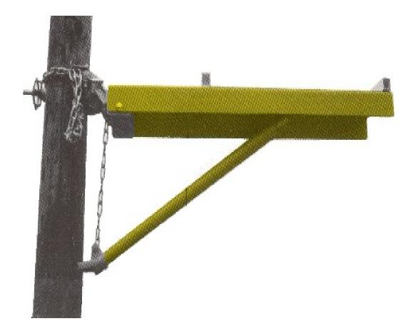
Baker boards are <u>not</u> considered a form of primary insulation. (just because you're standing on a baker board doesn't mean you can bare hand primary)
